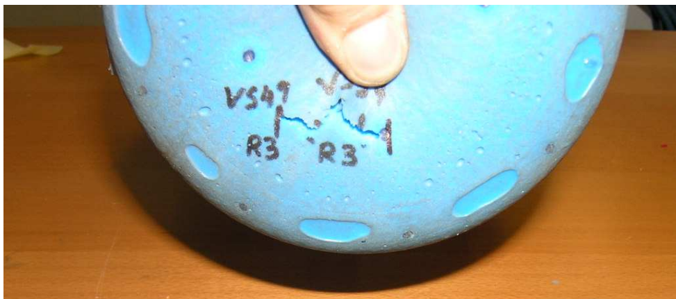
Fig. 3.3: Typical damage/crack after secondary impact of a high speed (55km/h) test.
