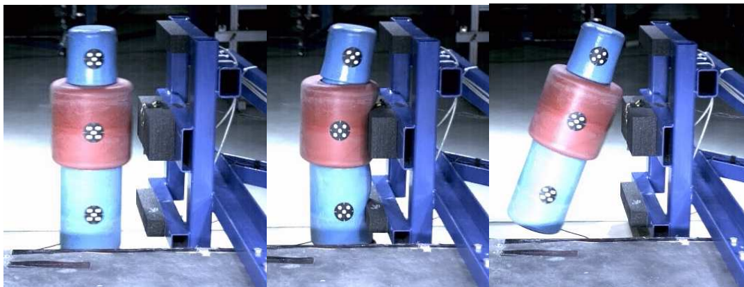
Fig. 3.1: PDI-sled-test at 20 km/h using a standardised vehicle frontend.
